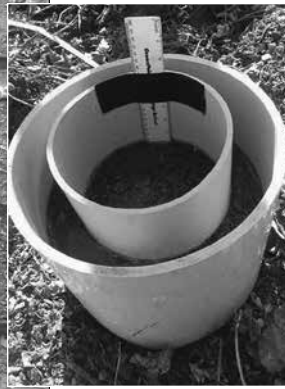
Infiltrrometer constructed from sturdy sewer piping with beveled bottom. Infiltrrometer is pounded into the ground, either by twisting it down or pounding a wood block with a sledgehammer, deep enough to ensure water enters soil and does flow out from the bottom onto the adjacent soil, usually 3-10 cm. Less durable infiltrrometers can be constructed from 5 gallon plastic buckets or large tin cans.
